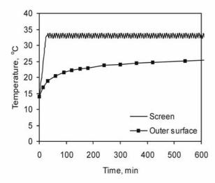
Fig. 3. Temperature variation of the screen and surface of the heated trap at 14.5 °C temperature of grain
